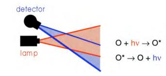
✓ Light scattering on ice particles at 121.6 nm
