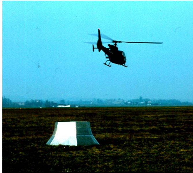
Fig. 2. A portable microphone shelter during a field test (photo L. Liszka).
