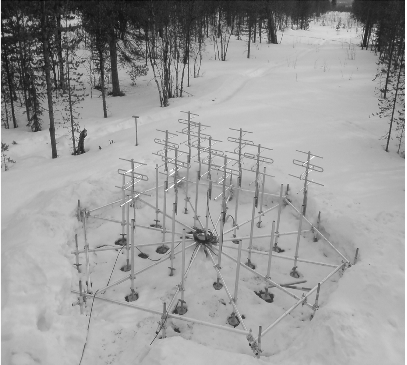
Figure 2. Photograph of the mutual coupling test stand with ten Renkwitz Yagi antennas installed.
