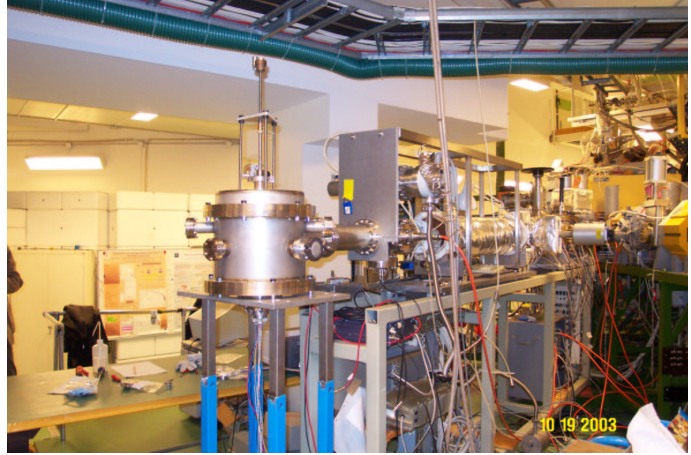
Figure 4.18: The Manne Siegbahn Laboratory CRYRING accelerator with a diameter of 30 m. The tangential 0° output with the NUADU calibration vacuum chamber on the end of a long drift tube is shown to the right.
