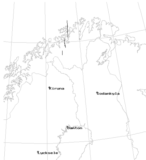
Fig. 36. The horizontal projection of trajectory segments determined at different frequencies (from N: 2.5, 3.5 and 4.5 Hz) combining Kiruna and Jämtön data.
