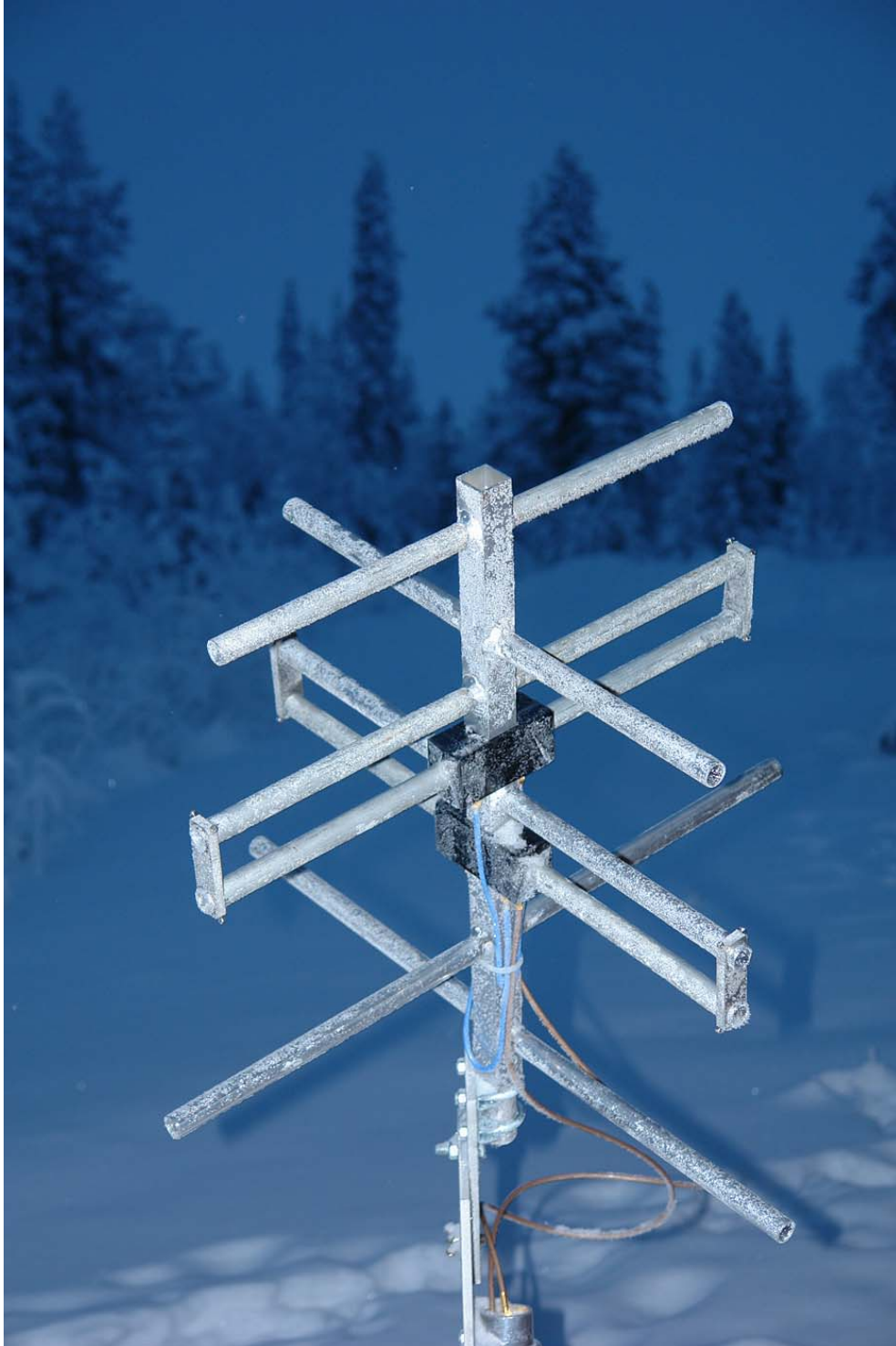
Figure 7: The first 235-MHz X Yagi, constructed to the mechanical specifications given in Table 1, under typical midwinter conditions. In this beta version, the folded dipoles are made with movable shorting bars to allow a limited amount of fine-tuning. The production run antennas will have their dipoles made from formed continuous lengths of aluminium tubing. The blue cables that are strapped down onto the boom are half-wave baluns transforming the nominal 200 ohm balanced feedpoint impedance to 50 ohms unbalanced.
