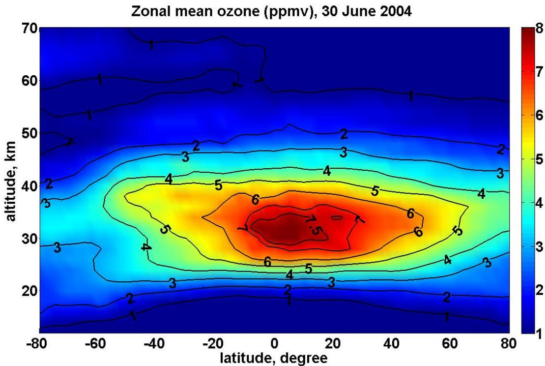
**Figure 5.** Latitude-height cross-section of the zonal-mean ozone volume mixing ratio (ppmv) obtained from the Odin SMR data for solstice conditions (30 June 2004).
