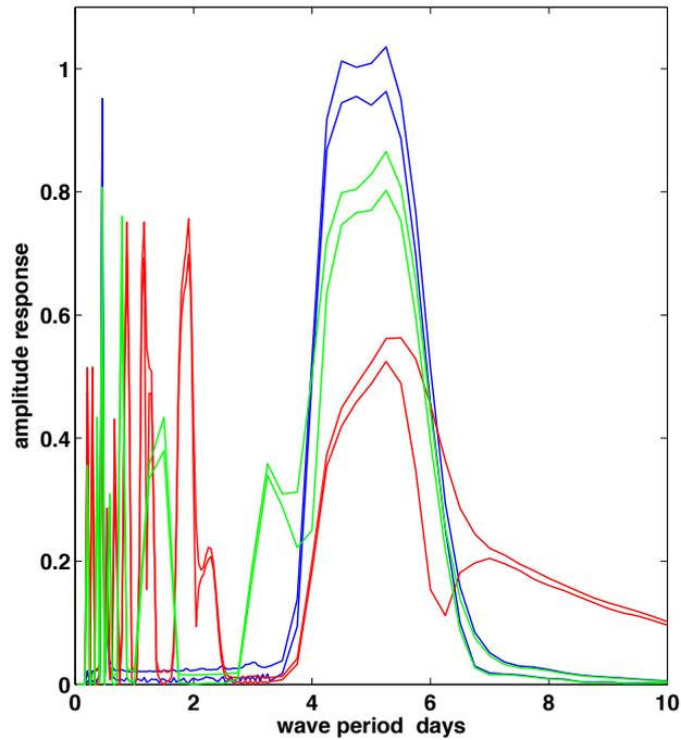
**Figure 11.** Amplitude response for the 5-day wave that has been obtained from simulated time series for waves with unit amplitude and different sampling schemes: blue: sampled at 12 h intervals; green: sampled at 2 consecutive 12 h intervals each 2 days; red: sampled at 2 consecutive 12 h intervals each 3 days.
