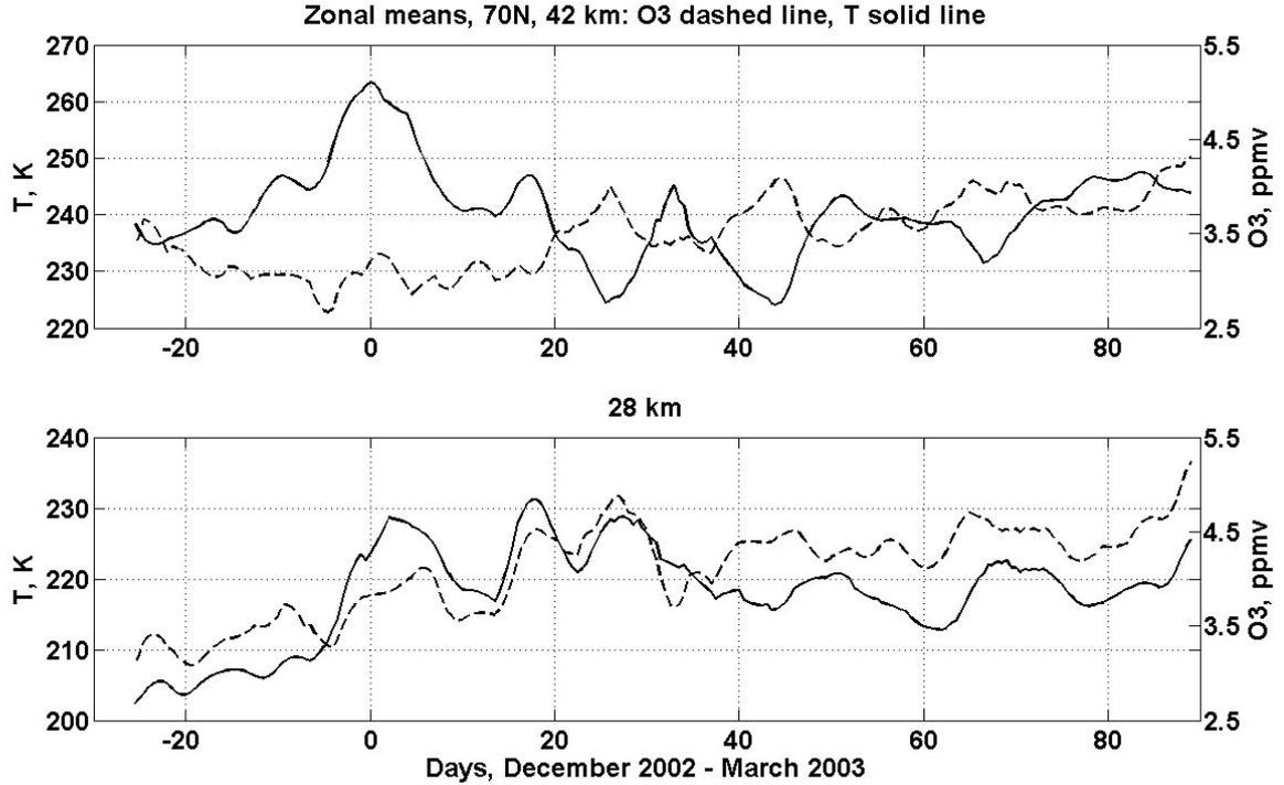
**Figure 6.** Zonal means from the Odin data for temperature (left scale, K, solid line) and ozone (right scale, ppmv, dashed line) at 70°N; upper panel is for the 42 km level, lower panel is for the 28 km level (Figure 3 from Paper III).
