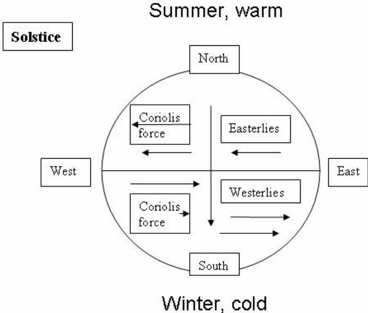
**Figure 3.** Schematic picture of the circulation in the stratosphere for solstice conditions, NH summer. Coriolis force deflects air flow to the right (west) in the NH and to the left (east) in the SH.
