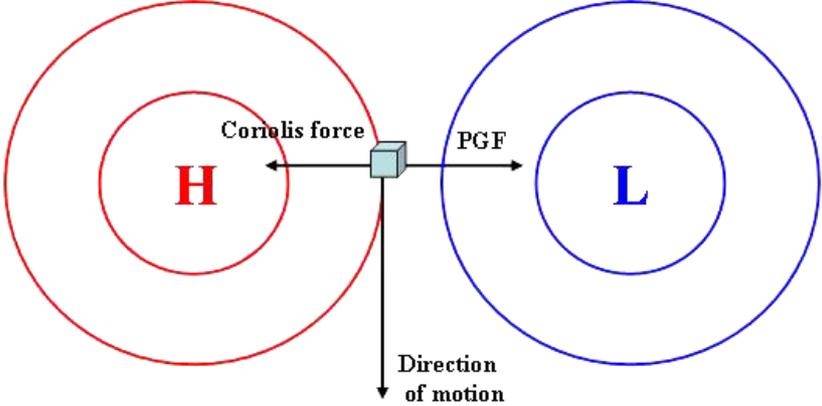
**Figure 2.** Schematic plot of geostrophic balance. In the upper atmosphere, above the friction layer, the friction force acting on an air parcel is practically negligible. Therefore, only two forces act on the parcel, Coriolis and Pressure Gradient Force (PGF). When these two forces balance each other, the situation is called the *geostrophic balance*. This balance leads to wind motions that circulate along isobars (surfaces of constant pressure) at a given height.
