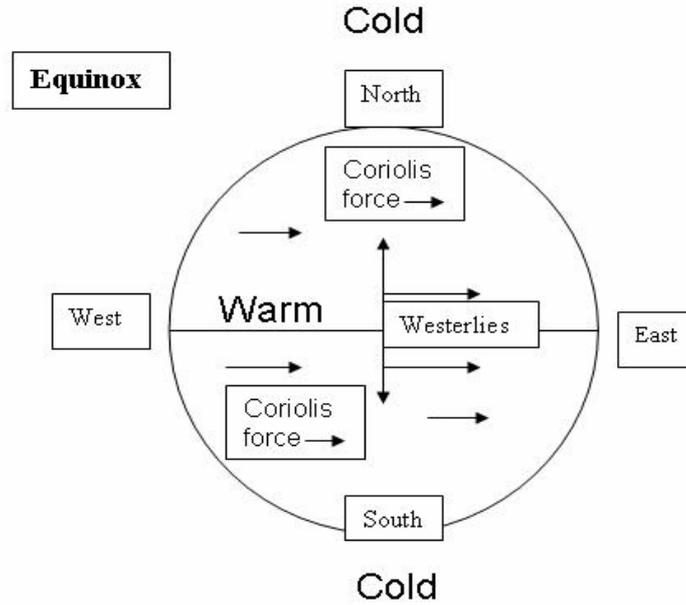
**Figure 4.** Schematic picture of the circulation in the middle atmosphere for equinox conditions. The pressure gradient is from the warm equator region to both the colder poles, and the winds are westerly in both hemispheres.
