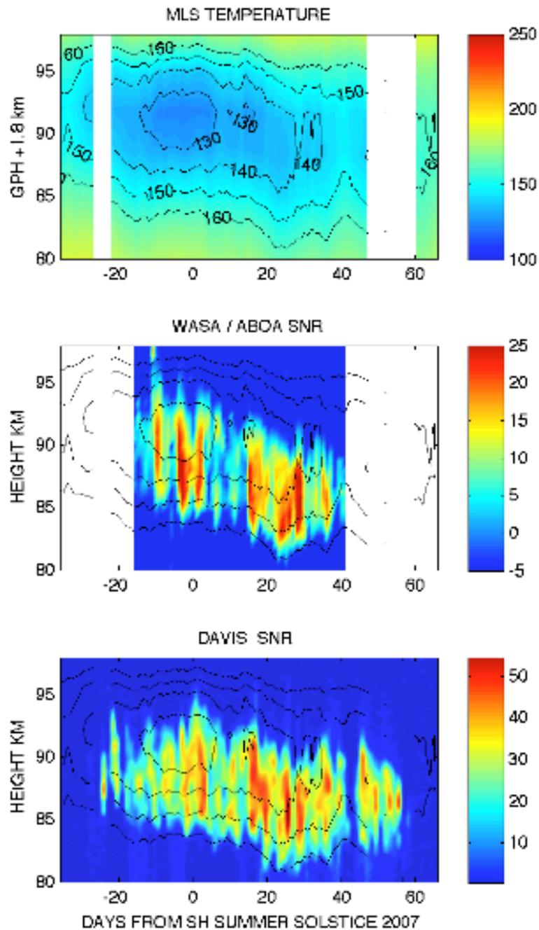
Figure 1. Top panel: Zonal mean temperatures from Aura-MLS averaged over latitudes 70-75 ° S. Middle panel: PMSE SNR (dB) measured at Wasa/Aboa. Lower panel: PMSE SNR (dB) measured at Davis. MLS temperature contours are reproduced on all 3 panels.
